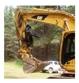
The PAKGRAPPLE is new technology that offers a unique solution to situations that require the versatility of a single machine needing to employ a bucket for excavation and tree removal as well as having a heavy duty grapple with saw available for tree and stump handling. The PAKGRAPPLE is foldaway, and can operate in the extended operation position without requiring removal of the bucket.
